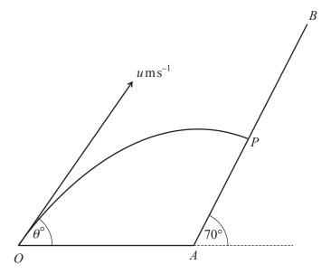
The diagram shows a surface consisting of a horizontal part OA and a plane AB inclined at an angle of  $70^{\circ}$  to the horizontal. A particle is projected from the point O with speed  $u\,\mathrm{m\,s^{-1}}$  at an angle of  $\theta^{\circ}$  above the horizontal OA. The particle hits the plane AB at the point P, with speed  $14\,\mathrm{m\,s^{-1}}$  and at right angles to the plane,  $1.4\,\mathrm{s}$  after projection.
